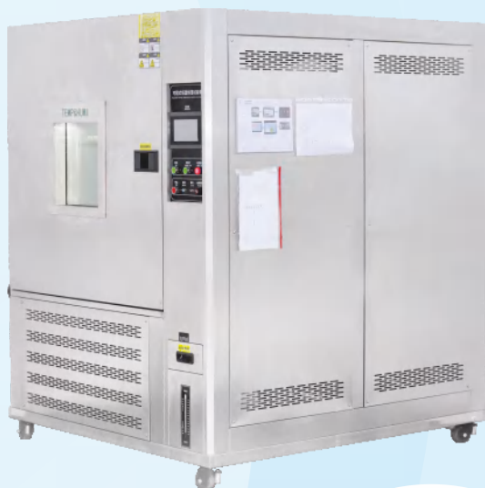
高低温循环老化测试 / High and low temperature cycle aging test
